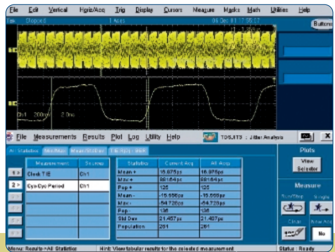
► Figure 12. This TDSJIT3 measurement screen includes several concatenated jitter measurements taken at 20 GS/s. It reveals a PLL signal that has almost 1 ns of error within a 7.5 ns cycle.
