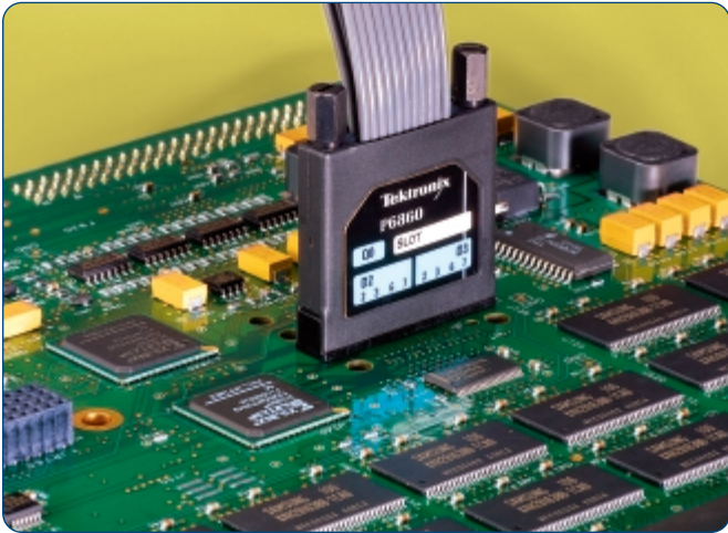
▶ Figure 4. The new HD compression analyzer probe architecture provides a simple connection that delivers clean signals from the system under test to the instrument.
